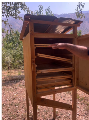
Figure 18: GIZ- designed dryer, shelves left reinstalled incorrectly
