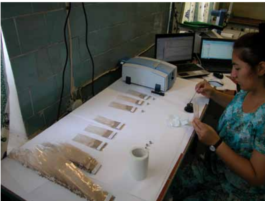
Soil spectral measurements facilitate monitoring of soil conditions, Tajik Soil Institute, Tajikistan (Johanna Zwahlen 2012)
